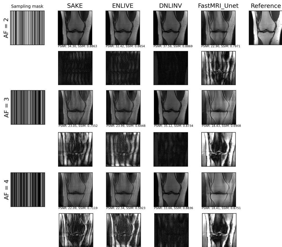
Fig. 6. Knee 1d calibrationless retrospective undersampling comparing SAKE, ENLIVE, DNLINV, and the fastMRI pre-trained Unet reconstructions. The absolute difference image are shown below each reconstruction and the error intensities were amplified by 3x to improve visibility. Even at the lowest AF = 2.0, only DNLINV is the only method largely free of parallel imaging artifacts. At higher acceleration factors. While some aliasing artifacts appear at AF = 3.0 and 4.0 in DNLINV, the error is still much smaller compared to the other methods.
